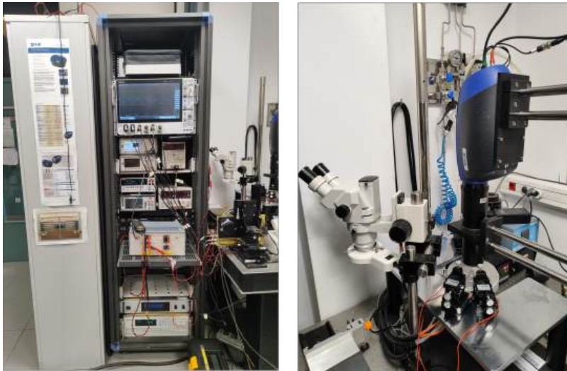
Figure 5.31: Infrared lock-in thermography setup present at CNM Barcelona.
