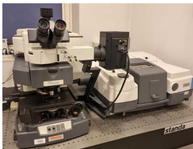
Figure 18. Measurement instruments - Thermo Scientific Nicolet 8700 spectrometer with the Thermo Nicolet Continuum microscope, on which the experiments were carried out.
