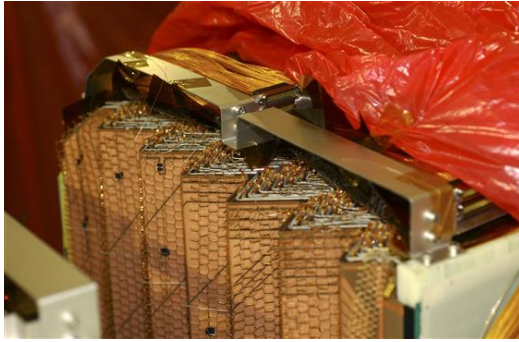
Figure 2.7: Characteristic accordion structure in EM calorimeter [64].
